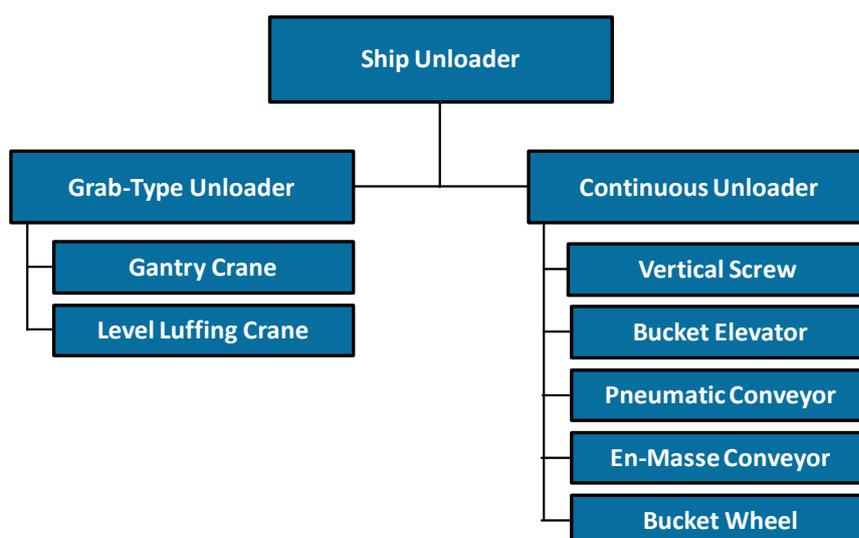
Fig. 5: Classification of different types of ship unloaders.
