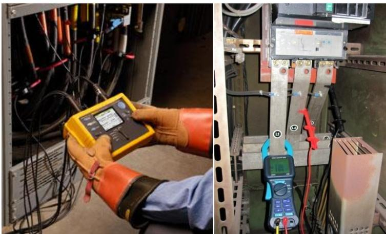
Fig. 8: Power meters to measure the consumption of driving units and whole systems.
