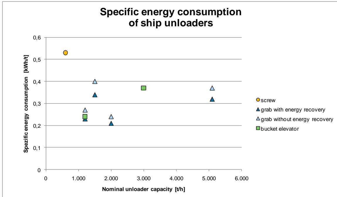
Fig. 15: Comparison of the specific energy consumption of all measured ship unloaders.
