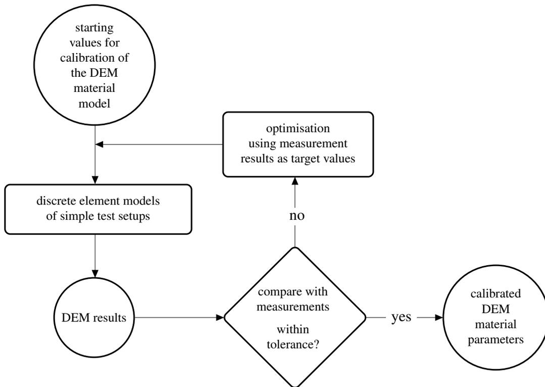
Figure 3: Optimisation procedure for DEM models
