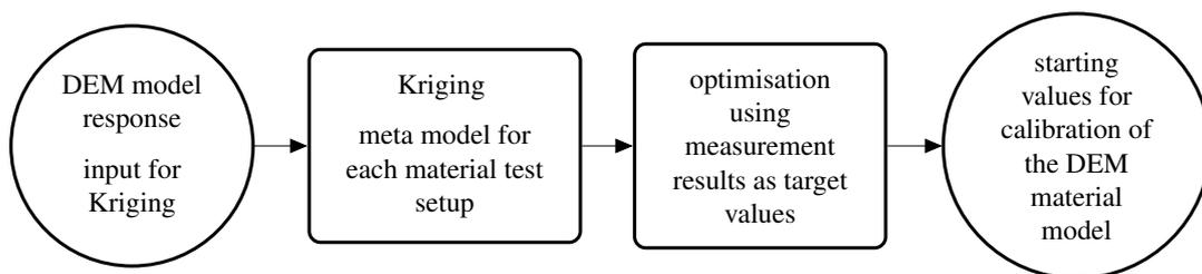
Figure 2: Response data from the LHS are used as input to the Kriging models.
