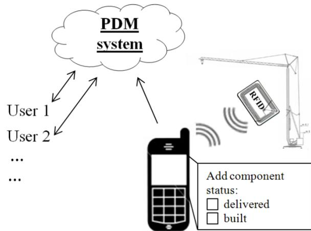
**Figure 2** Concept of the construction progress control system
