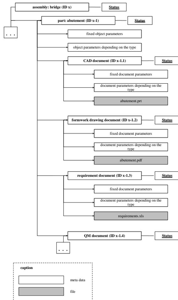
Figure 4 Ontology of a PDM system customized and enhanced for the construction industry [10]
