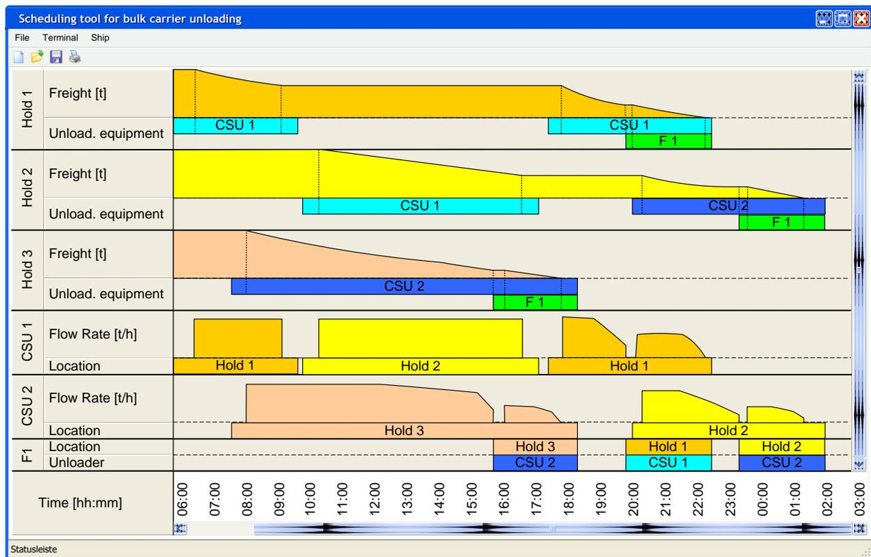
Fig. 5: Mock-up of the auxiliary tool for planning the unloading procedure (CSU: Continuous ship unloader; F: Feeding device)
