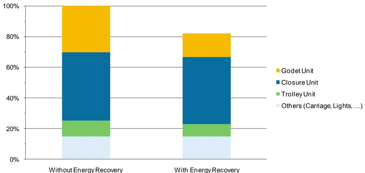
Fig. 4: Breakdown of the Power Consumption of a Gantry Crane with and without Energy Recovery
