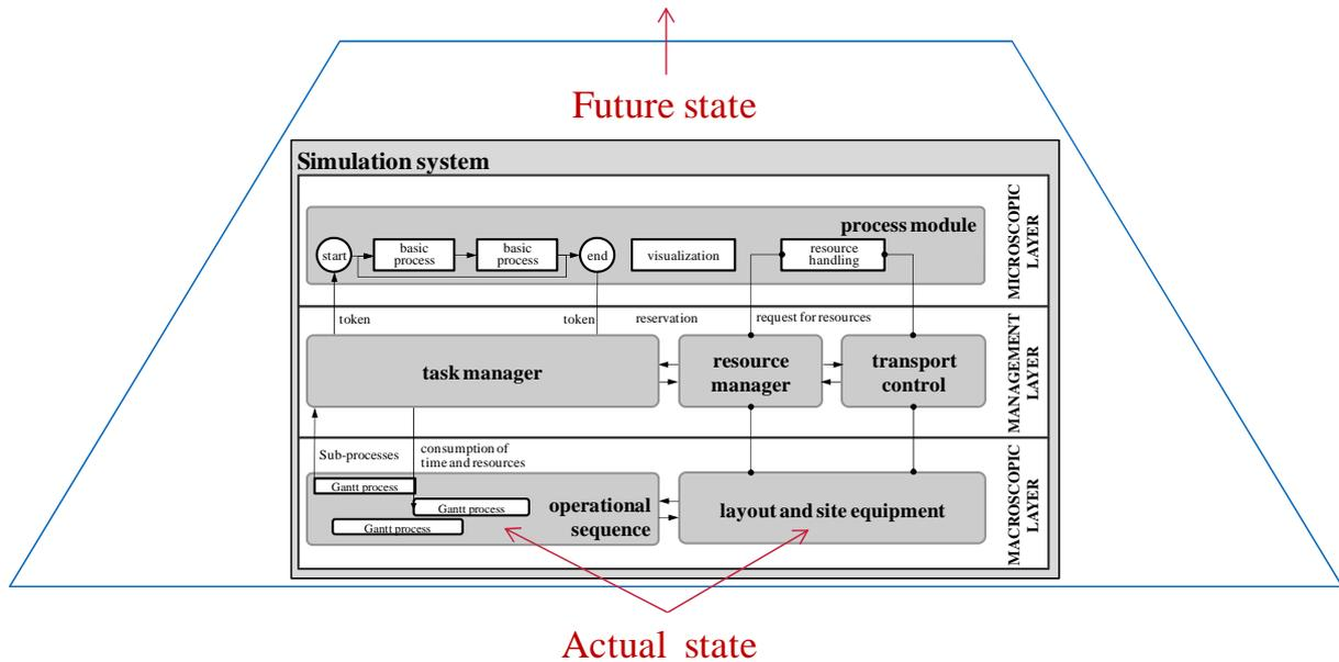
Figure 3: Internal interaction of the different modules in the detailed process simulation
